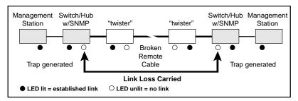
**IMPORTANT:** When connecting a "twister" 2131 media converter to a port that supports auto-negotiation, it is strongly recommended to fix the port setting to the appropriate speed (100Mbps or 10Mbps) and to either full or half duplex. This allows the media converter to sense receive link and select the active port.
