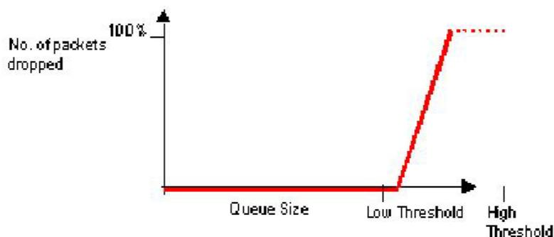
On the layer 2 card the maximum drop probability is  $maxp=0.1=10\%$ , this is different compared to Ethernet mapper cards, where the maximum drop probability is  $maxp=1=100\%$ .
