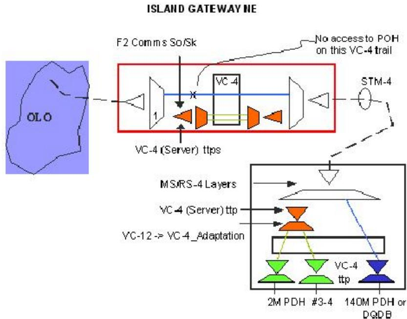
An Island Gateway NE operates as a 'tail-end' node for F2 communications with conversion back to SDH OH DCC.
