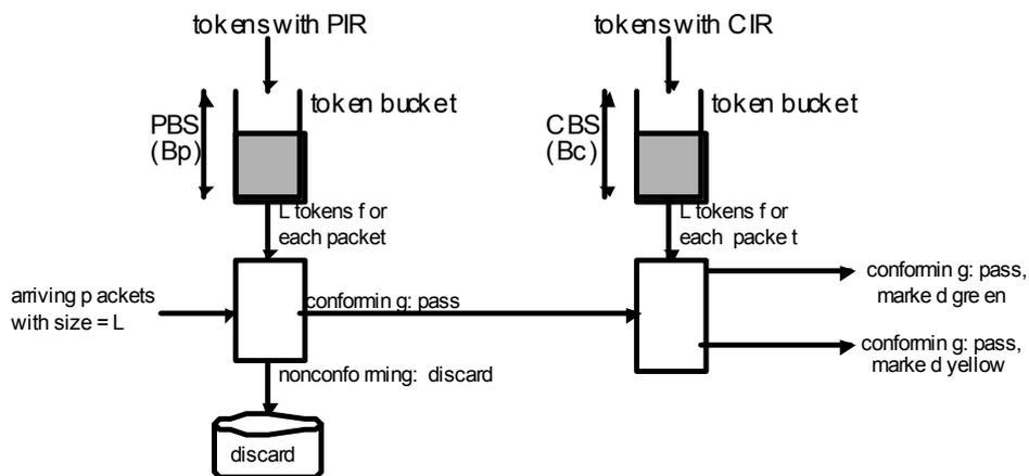
The first token bucket monitors the PIR (measured during an interval of PBS). If PIR or PBS is exceeded, the trTCM discards those packets. The second token bucket monitors the CIR (measured during an interval of CBS). The trTCM marks packets, which are in conformance with CIR and CBS as green, packets, which are not in conformance with CIR, and CBS as yellow.
