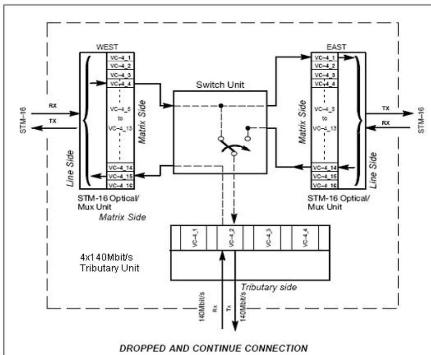
In the example illustrated in Figure 6-14, the channel VC4\_4 (UCD Worker) incoming to line West is unidirectionally connected to channel VC4\_1 outgoing from line East, it is also unidirectionally connected to VC4\_2 outgoing from the tributary unit.
