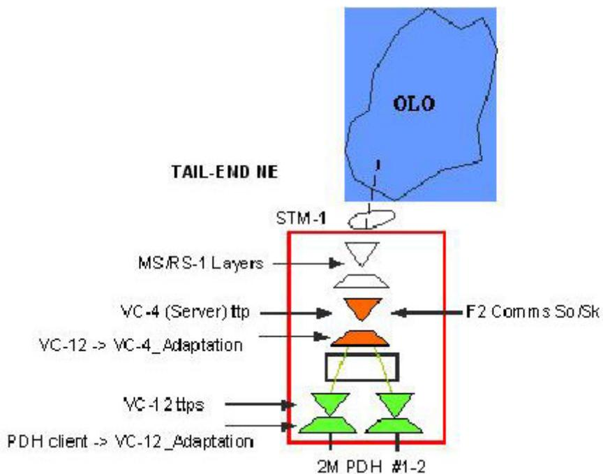
An isolated 'Tail-End NE' type operates as a 'tail-end' node for F2 comms.
