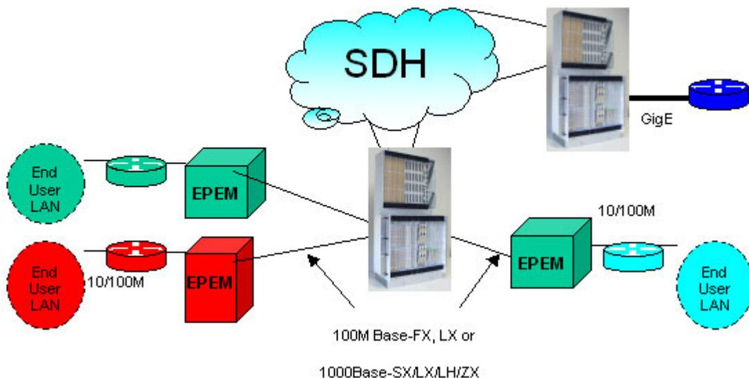
The EPEM provides a client port to the end user, and a WAN port for the optical fibre connection to the Ethernet card.
