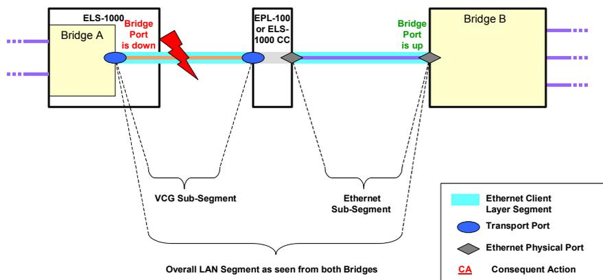
Figure 6-11 presents a scenario in which the MAC layer is not contiguous, i.e. the failure of the MAC layer on the VCG sub-segment is not propagated to the Ethernet sub-segment. As a consequence, Bridge A regards its connected port and hence the whole segment as not operational, while bridge B regards the segment as operational. This results in inconsistent topology information being used by the bridges and consequently the calculated active topology will be erroneous.
