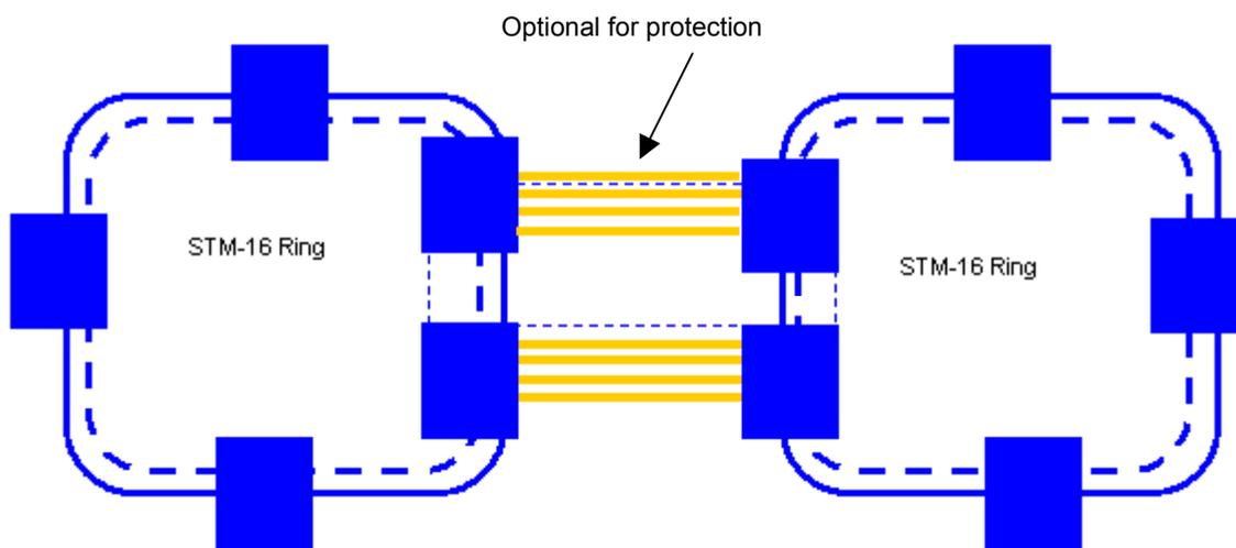
Replacing the traditional existing SDH Multiplexers by Marconi OMS 1600 saves on the cost of the second interconnection multiplexer, the interfaces between both multiplexers, and reduces the possibility of errors, the required space, power consumption and cost. Additionally it reduces the numbers of managed network elements and the effort needed to reconfigure for an increase in interconnection traffic.
