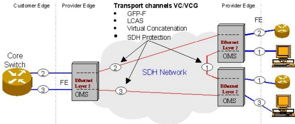
Figure 6-1 shows a network providing the EPL service. The SDH transport network connects Ethernet ports on each side of the network. Each of the private lines (1) to (3) is completely separated, which means there is a port per customer on each side of the network. The ports are connected via separate SDH transport container groups. That is no say no aggregation of Ethernet flows is taking place.
