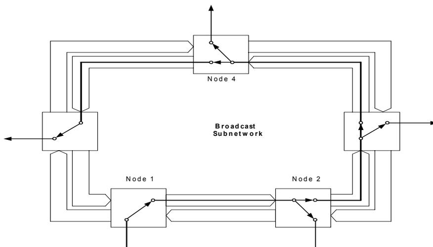
Figure 6-14 shows a Point-to-Multipoint Unidirectional Cross Connections at a single node.
