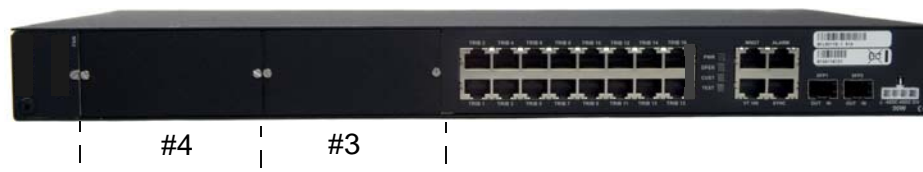
Figure 6 Service modules - Slot positions
