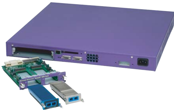
Summit 400 with optional Summit XEN 10 Gigabit Ethernet module and two XENPAK I/O modules
