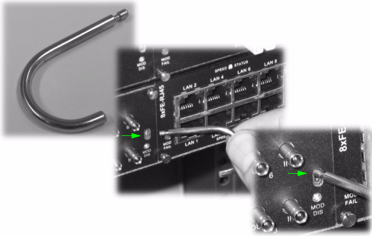
Figure 1-8. Remove module using the Card Extraction Tool
