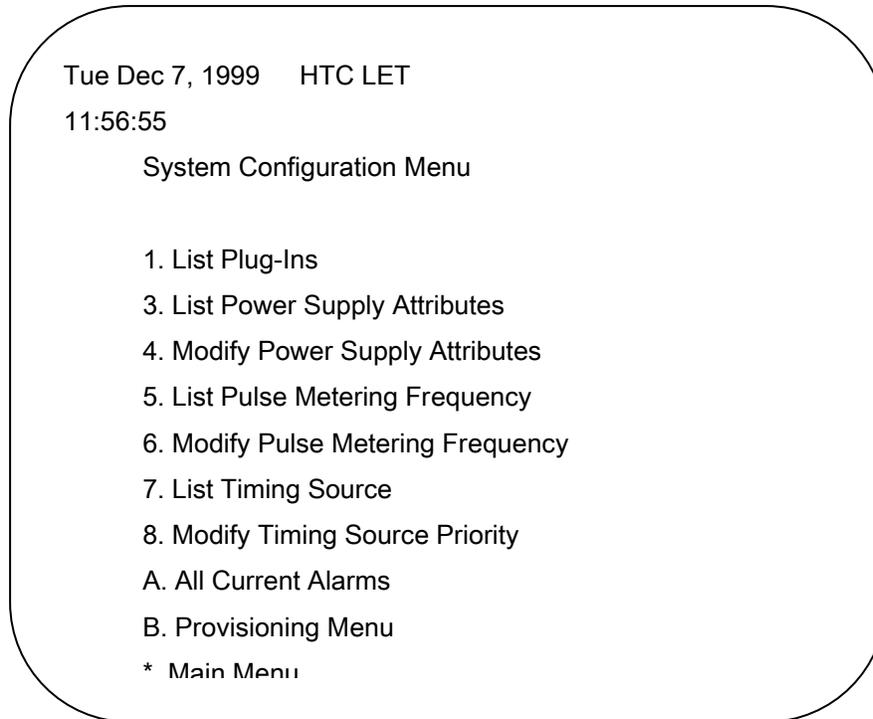
**Figure 3-b. The System Configuration Sub-menu**
