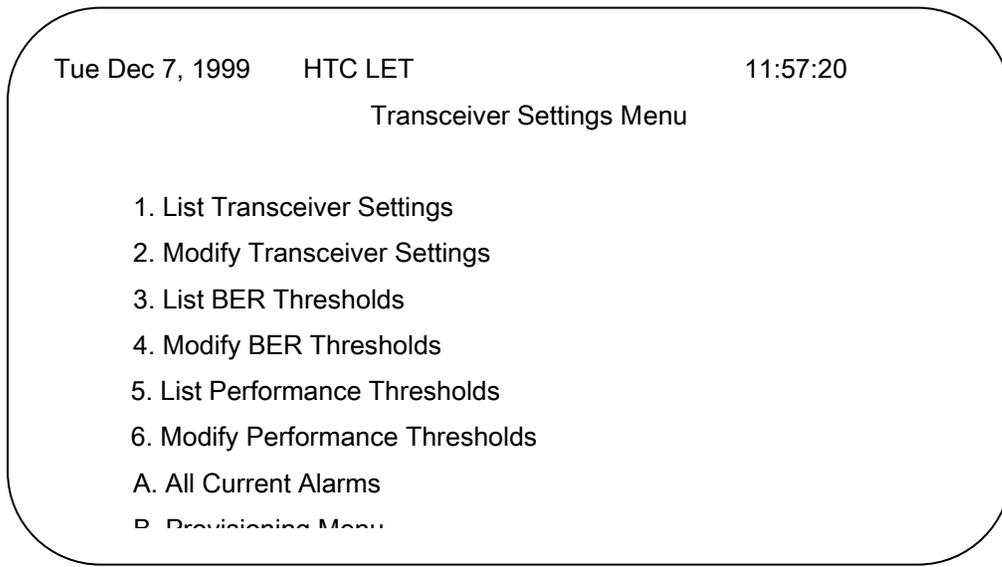
**Figure 3-j. HTC-1100E Craft Interface Transceiver Settings Sub-menu**
