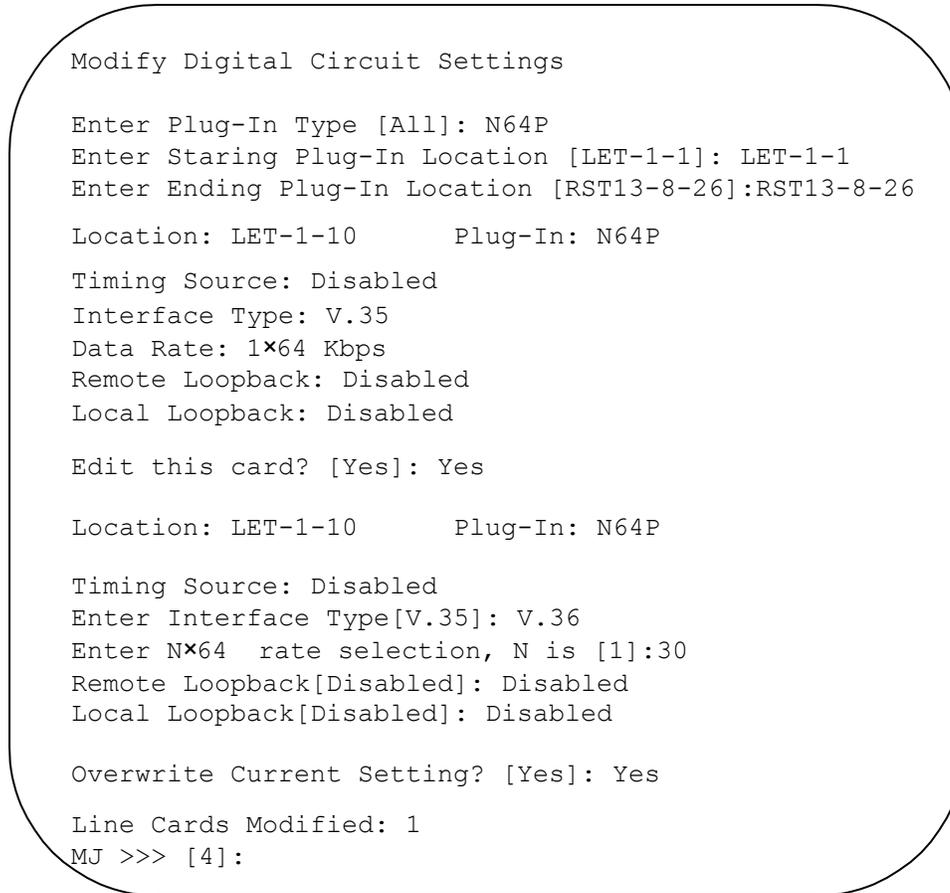
**Figure 3-s-5 Sample Screen of N64P**
