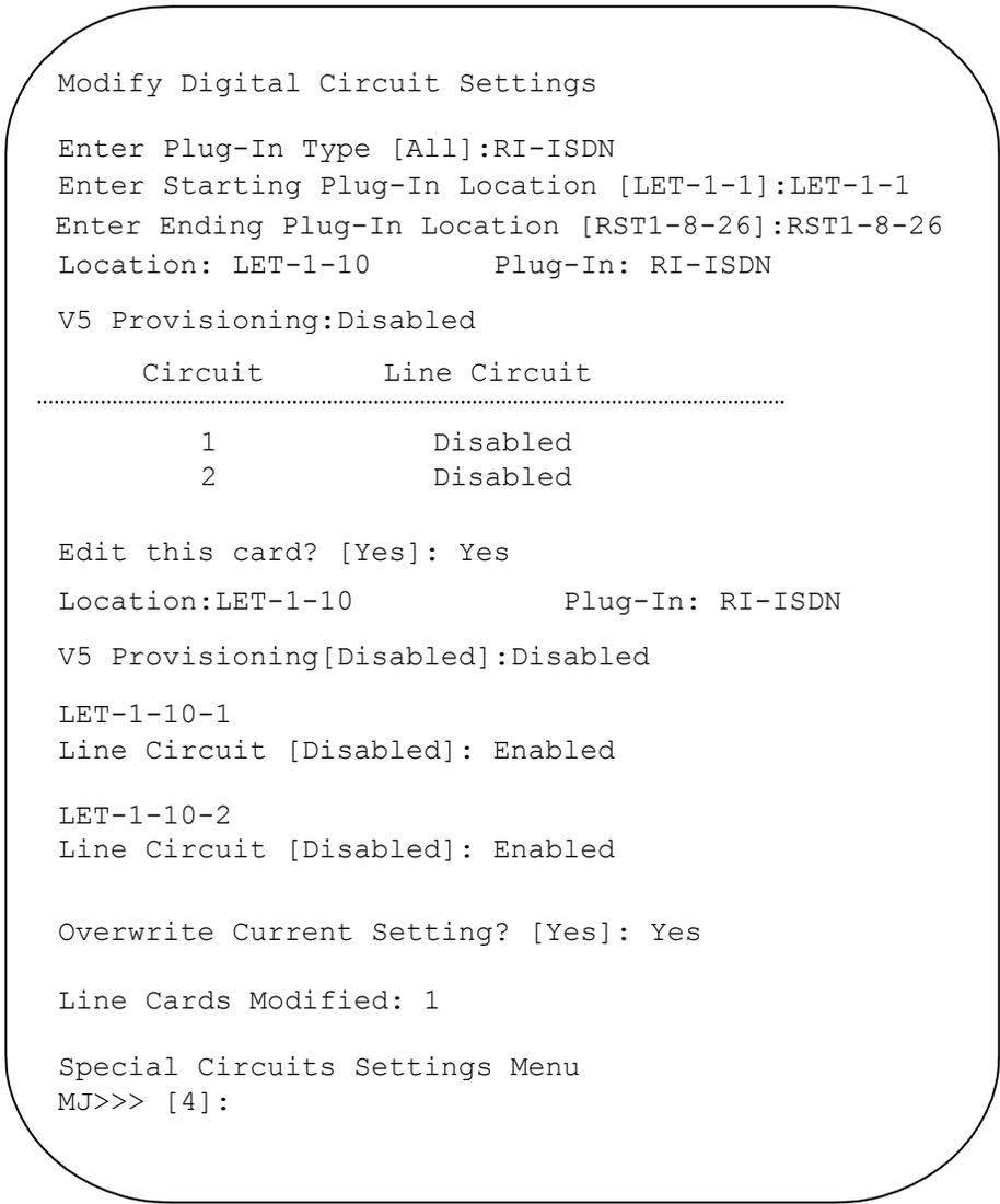
**Figure 3-s-7 Sample Screen of RI-ISDN**
