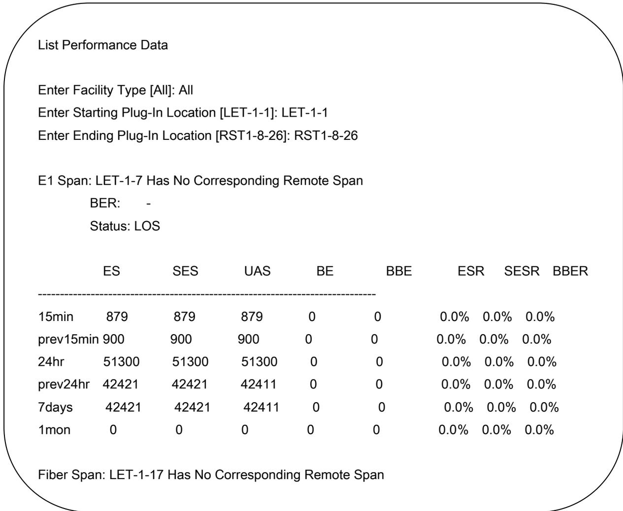
**Figure 4-e. Sample Output of List Performance Data Command**
