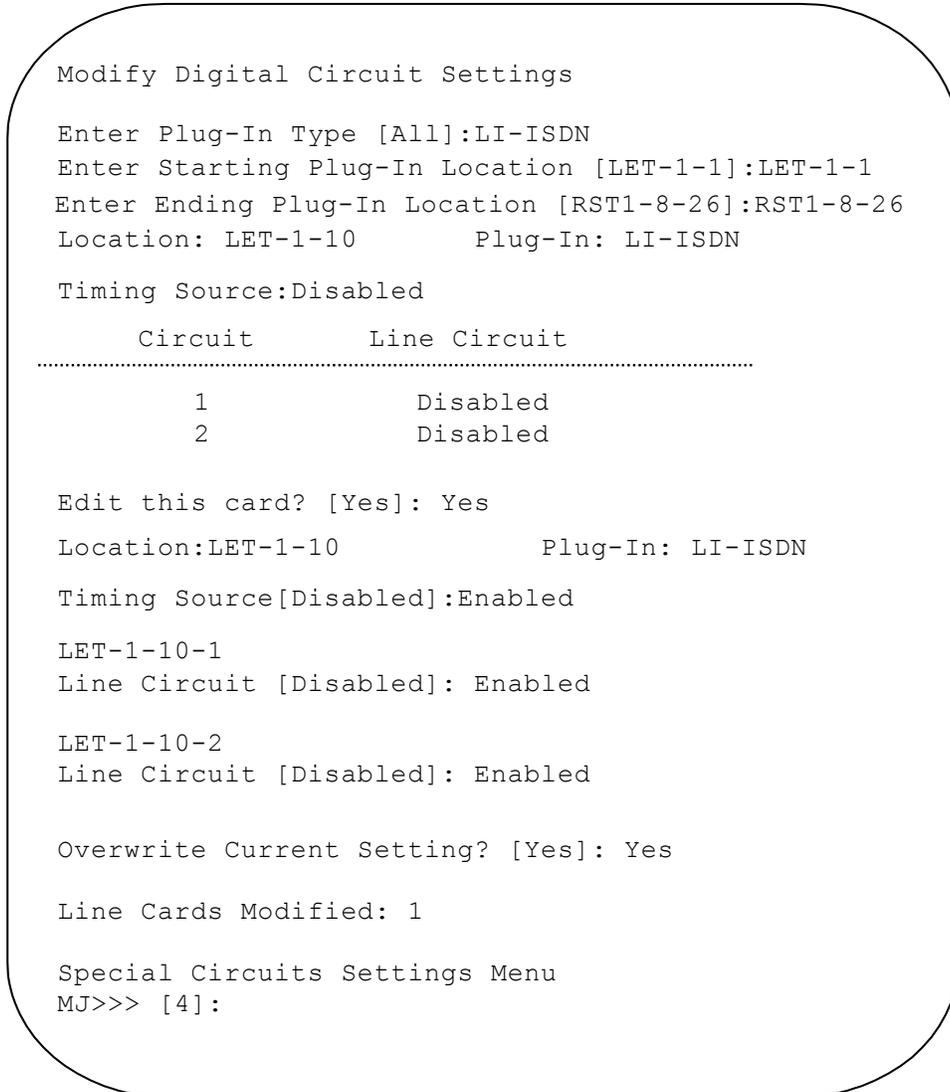
**Figure 3-s-6 Sample Screen of LI-ISDN**
